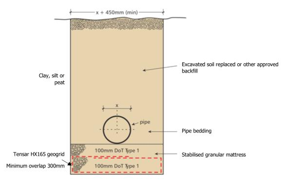
The efficient interlock mechanism between the HX165 geogrid and aggregate creates a flexurally stiff supporting mattress which provides an effective load spread into the weak ground, and also helps to mitigate, but will not eliminate, any longitudinal differential settlement which may start to take place.
